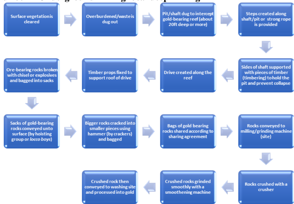
Figure 16 Steps in Underground Mining
