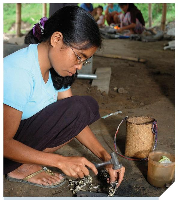
**Traditional brass making** — Lake Sebu, South Cotabato. Once the clay mold is broken, the brass casting can be processed. Individual bells are hammered out of the "brass tree". (ILO/A. Barredo, August 2009)
